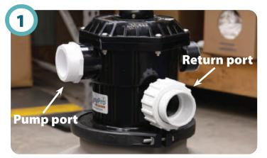
Open filter box, follow the enclosed instructions. Attach the union to the return port on the filter and the half union on the pump port. DO NOT OVERTIGHTEN!
