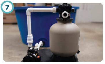
Place the filter on the equipment pad. Line up assembly #4 from the pump's outlet to the pump port of the filter.
