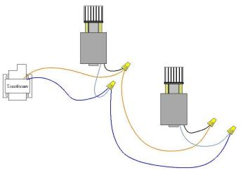
The Vulcan Fire Modules have a Yellow and a Blue wire protruding from them. These are the power wires.
